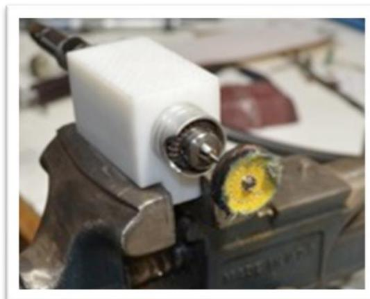
**Step 2.** Put on safety glasses and a particle respirator. Start the flex shaft and run the edge of a piece of metal across the face of the buff. This is called “dressing the wheel.”
