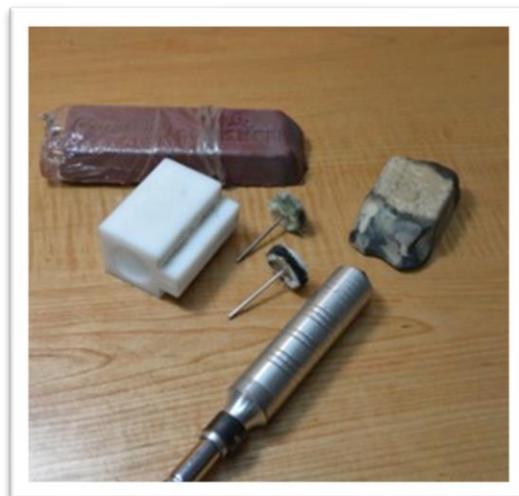
**Step 1.** Secure the flex shaft handpiece in the handpiece holder, ensuring the rotation is down and away from you. Attach a mandrel with a yellow-treated buff to the handpiece.
