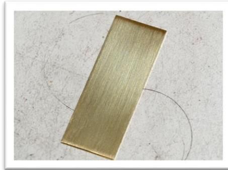
**Step 2.** Using the next finer grit sandpaper—600 grit—turn the piece of metal 90° and begin sanding against the grain. The previous scratches begin to disappear, and a finer set of scratches take their place. Continue this until there is a uniform 600-grit scratch surface.
