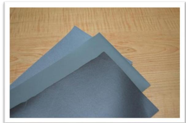
The grit of sandpaper that you start with will depend on the severity of the scratches on the surface of the metal. With experience you will know what to start with. Rinse the metal often to check progress, and always rinse the piece well. Wipe off any excess moisture before progressing to the next step. The second photo shows the uniform 400 grit scratch surface.
