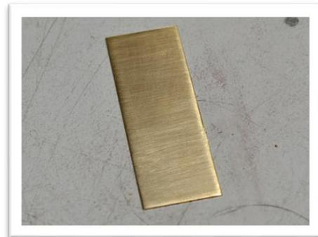
**Step 3.** Repeat steps 3 and 4 with finer and finer grit sandpapers. When using a polishing lathe or a flex shaft with buffs and compound, it's not usually necessary to go finer than 1200 grit.
