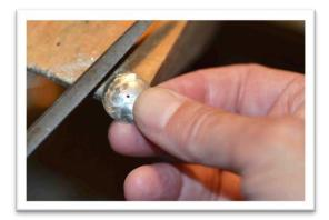
In later projects, you can leave the coin's original surface intact, or remove it and sand the surface with 220, 400, 600, 800 and finer grades, finishing it to a high polish. Use flexible salon nail files from a beauty supply.
