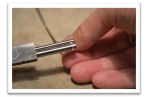
The Wubbers Bail Making Wubbers 3.0, 5.0 mm pliers make this task easy. Just be sure to make the bail *slightly* larger than the stone.
