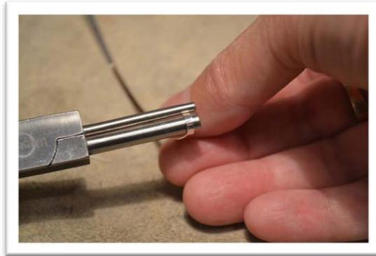
The Wubbers Bail Making Wubbers 3.0, 5.0 mm pliers make this task easy. Just be sure to make the bail *slightly* larger than the stone.
