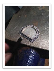
Flip the piece over and use the rectangular wire to make a frame around the assembly.
