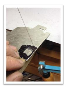
Drill the resulting shape, trace a rim of about 2mm all the way around, and pierce it as well. This will result in a frame where the stone will sit in later stages.
