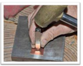
**TECH TIP:** Using a brass mallet, which is made of a relatively softer metal, is easier on your stamps and also prevents the mallet from glancing off the stamp.
