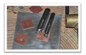
**Step 5.** Using the Steady Stamp jig and placing a piece of scrap the same gauge as the piece we're stamping on under the back of the jig, this large stamp can be used with confidence!
