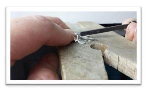
Place the bezel pusher so you can push the bezel onto the face of the girdle, using a rocking motion. Continue all of the way around the stone.
