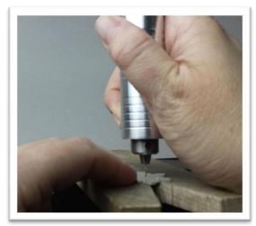
**TIP:** It is important to start with a small (pilot) hole first, then gradually use larger bits. Otherwise, the bit may grab the metal and possibly turn your snowflake into a throwing star. Even while doing it gradually, make sure you have a very secure grip on the piece (or clamp it) when using the largest bit.
