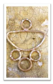
Light the torch and warm the assembly to dry the flux to a white powder. Once the flux is dry (white powdery), move the torch closer and apply more heat to the link. Keep the torch moving slowly. The flux will begin to change color. When the flux looks like dark syrupy caramel, the solder will flow. A bright silvery flash of flowing solder will appear in the seam between the "D" link and jump ring. Remove the heat quickly to prevent the solder from over-flowing.
