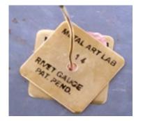
**3.** Place a #14 Rivet Gauge<sup>†</sup> on top, aligning all the holes. The #14 Rivet Gauge<sup>†</sup> is used on top, resulting in a longer stub of wire to accommodate the bezel cup and still allow the formation of a solid rivet within the bezel cup.
