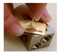
**2.** Place the assembly on the bench block, with the head of the ball rivet resting on the bench block and the wire tail sticking up into the air. Place the Rivet Gauge<sup>†</sup> over the wire and rest on top of the assembly. Use index finger and ring finger to stabilize the assembly on the bench block.
