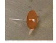
Place the ball rivet through the pieces to be riveted.
