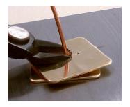
**6.** Remove the Rivet Gauge<sup>†</sup>, exposing the stub of riveting wire. Tap the exposed end of the rivet wire with a riveting hammer or the peen side of a chasing hammer to flare and form the first side of the rivet.
