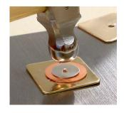
7. Invert the stack so that the remaining Rivet Gauge<sup>†</sup> is on top and the previously formed rivet head is on the bottom, against the bench block. Remove the remaining Rivet Gauge<sup>†</sup>, exposing the stub of riveting wire. Tap the exposed end of the rivet wire with a riveting hammer or the peen side of a chasing hammer to flare and form the final side of the rivet. The rivet is complete.
