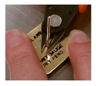
**3.** Using middle finger to control wire tail, with the flat back of flush cutters resting on top of the Rivet Gauge<sup>†</sup>, snip-off the rivet wire flush with the Rivet Gauge<sup>‡</sup>.
