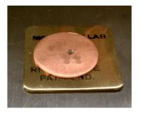
**5.** Remove the top Rivet Gauge, texposing the stub of riveting wire.
