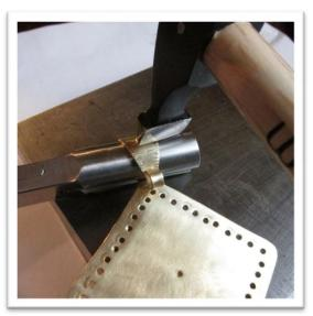
Using the bench block and the pliers as support, gently texture the piece using the WUBBERS Artisan's Mark Sharp Texture Hammer. (*the entire piece could be textured prior to forming the bail, but I didn't decide to texture until this step.*) Proceed to texture the entire front surface, if desired. I left the curlicue element un-textured for contrast.
