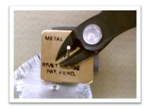
**SAFETY TIP:** ALWAYS wear safety glasses when cutting wire and metal—small pieces of wire or metal can fly into unprotected eyes.
