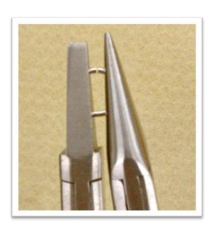
**Step 36.** Twist the pliers away from each other to open the jump ring like a gate.
