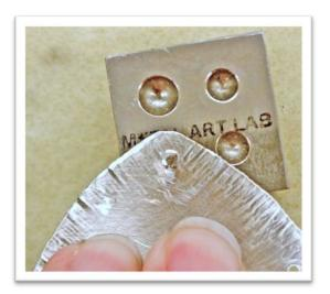
**Step 31.** The corner rivets are completed first. They have a lower profile than the center assembly. When planning the order of rivets to complete, the lower profile rivets are completed first.
