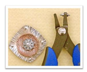
**Step 34.** Place the punch of the hole-punching pliers on the remaining mark on the silver piece. Gently squeeze the handles of the pliers. The punch will "pop" through the metal, making a hole for the bail.
