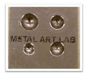
**Step 26.** Invert the piece and place the ball-head in one of the small cavities of the tiny dapping block. Use the smallest cavity that accommodates the head of the rivet. This will help stabilize the piece. There should be a small amount of space between the top of the dapping block and the face of the piece. This will prevent any marring of the piece when the rivet is set.
