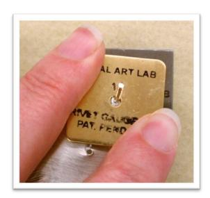
**TECH TIP:** Riveting Essentials Rivet Gauges<sup>†</sup> come in pairs and are marked with the wire gauge to which they correspond. Only one of the pair is used with ball-head rivets. Rivet Gauges stamped with a 14 are to be used with 14 gauge rivet wire, those stamped with 16 are to be used with 16 gauge rivet wire and those stamped with 18 are to be used with 18 gauge wire.
