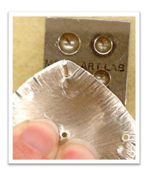
**Step 27.** Place the corresponding Riveting Essentials Rivet Gauge<sup>†</sup> over the tail of the rivet and hold the assemblage of pieces in place, stabilizing the pieces with two fingers.
