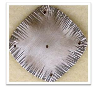
**Step 20.** Place the silver piece on the bench block. Place the sharp tip of the center punch on the center mark. Tap the opposite end of the center punch with the utility/household hammer to create a small divot in the metal. Repeat for all the remaining marks.
