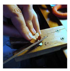
One option for sanding in tight places is to cut a thin strip of 60 micron sanding film and threading it through an old saw frame. This method is very effective for getting the spaces between the petals.
