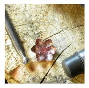
Another method is to use a hard, vulcanized rubber bench block with either a steel or a wooden dapping punch to round the petals. There will be less of a ruffled appearance, but the rubber block forms the petals nicely.
