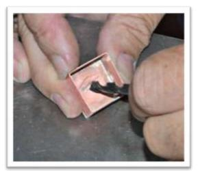
**Step 8.** After you've soldered the end on, take the jeweler's saw and trim the excess off. Don't file yet.
