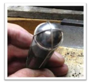
**Step 8.** Using the dapping punch, a nice curvy earring bottom is created and soldered together at the intersection using medium solder.
