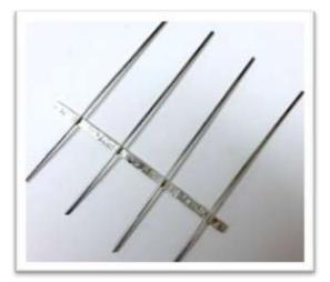
**Step 5.** The wires are soldered using medium solder. Quench, pickle, and rinse.
