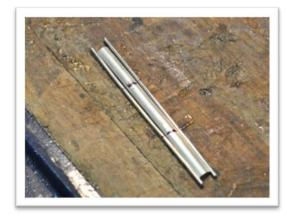
**Picture #12:** Using a pair of half round/half flat pliers, bend both 16 gauge wires on your marks so that when you solder them to the center piece, you'll only solder them in the center third. Don't worry if the bends aren't even, all that matters is that they are in the same place on both pieces.
