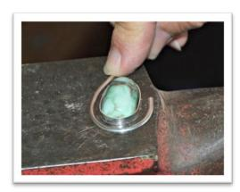
**Picture #5:** After you solder your joint with hard solder, pickle and rinse and then file the joint smooth to remove any trace of a joint. Finally, set it around your bezel to make sure it fits the way you want and hasn't lost its shape.
