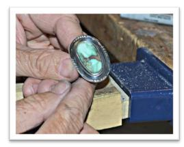
**Picture #18:** Use a burnisher to push the bezel around the stone. Start at the ends and work the bezel down over the sharpest curves on the stone and then finish off the middle sections. And there you have your finished ring.
