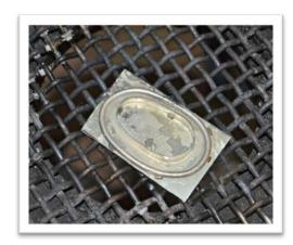
**Picture #8:** When you get your piece dried off, check to make sure your solder flowed into every area. When you're sure you have good joints, use a jeweler's saw to trim the excess plate. Saw close to your shadow box, but not into it. Leave a little bit to file off. Once its filed, clean up any flashing on the side/bottom of your plate with a fine cut file, and then sand the edge to make sure its smooth. Remember, jewelry isn't supposed to HURT!
