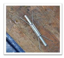
**Picture #14:** Put flux on your pieces and then put a couple of small pieces of medium solder on both sides of the center piece. I'm using medium solder because we'll be soldering two small 16 gauge pieces to one BIG 6 gauge piece, and I don't want to have to get my metal any hotter than I have to thereby reducing the chance that I'll melt one or both of the 16 gauge pieces while trying to get my solder to flow. Go ahead and solder, pickle and rinse.
