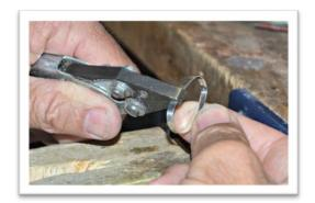
**Picture #3:** Apply flux to your joint, then put a small piece of hard solder over the joint. Start with a soft flame on your torch to slowly dry the flux, or else your solder will fly off into space. Once the flux is dry, turn up your torch and heat your joint evenly until the solder flows. Remember, solder will always flow towards the heat, so heat both sides of your joint evenly. Pickle and rinse.
