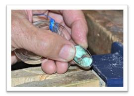
**Picture #2:** You must also make sure your bezel fits side to side with no twisting. I like to take my parallel jaw pliers and grab the joint, and then move the bezel up and down on time to take any of the fight out of the metal, and also insure that my joint is perfectly aligned on all axis.
