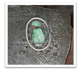
**Picture** #6: Set your bezel and shadow box on your sheet silver, which will become the backing plate. Use a Sharpie marker to mark your silver and then cut out the backing plate, using either shears or a jeweler's saw.
