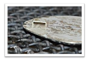
**Picture #20:** With the bail secure, I wanted to scuff up the bright, shiny bezel. I used a 36 grit 3M wheel on the flex shaft, but you can do this by hand.
