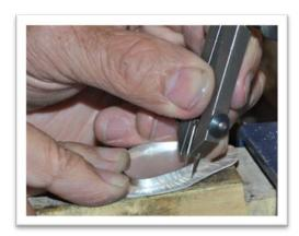
**Picture #17:** In order to make the pendant hang evenly, mark the top and bottom centers on the face where you can see where the true centerline is. If you're tempted to put your stone in the bezel to see how it will look, (and I highly DON'T recommend it) put a piece of dental floss under the center of the stone with a generous amount hanging out on either side so that your stone won't get stuck.
