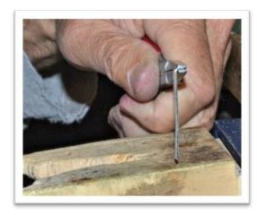
**Picture #15:** Making sure the space would be wide enough for the collar to pass through, in this case about 5/16" of an inch, bend the other side. Now cut off the long tail to match the other side and file flat.
