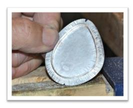
**Picture #18:** Flip you pendant over and transfer your marks to the back side and draw a line between them. You now have the center of your pendant so you can place your bail correctly.
