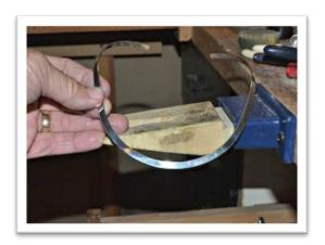
**Picture #13:** I started my bail by taking a scrap piece of 22 gauge silver, using my dividers and scribing a ¼" wide line so I can cut out a strip to form my bail with. I textured one side with my magic rock so it would match the rest of the back.
