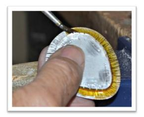
**Picture #23:** Place your stone in the bezel and push the bezel over the stone with a burnisher. Be careful not to scrape the burnisher over your nice patina. If you do, you should be able to sand out any minor damage.
