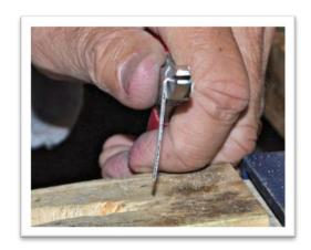
**Picture #16:** Using a pair of dividers spaced about ¼" apart, scribe a line around your bezel. Put one side of your dividers inside the bezel and use that as your guide. Now cut out along your scribe line with a jeweler's saw. File the edge, then sand with 400 grit sandpaper.
