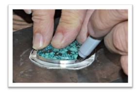
**Picture #8:** By striking the metal at an angle with the riveting hammer, we get a nice line impression. You could achieve the same look with a line stamp, but this is a little easier and faster. Once you've textured all the way around the piece, you're ready to texture the back with my exotic texturing tool.
