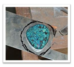
**Picture #4:** With your jeweler's saw, cut out your rough shape. Sand front and back with 400 grit sandpaper.
