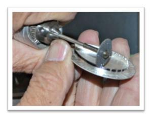
Picture #22: To get a nice color on the metal, I painted the piece, front and back, with liver of sulfur gel. If the color is a little slow in developing, you can gently heat the piece with your torch. This will literally take about 10 seconds. Rinse and give it a good going-over with your brass brush. The brass brushing will give you a nice sheen on the metal. After brass brushing, dry your piece off and sand it front and back with the 600 grit sandpaper to bring out the textures.
