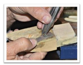
**Picture #14:** Take flat-nosed Wubbers and make a right angle bend on one end of your strip, leaving a tail about 1/8" long.
