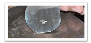
**Picture #7:** We're going to texture the front of our pendant with a riveting hammer. So we don't have to texture more than necessary, mark the outline of your stone with the bezel on. Be sure to center the stone before you mark the plate.
