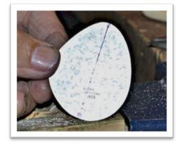
**Picture #19:** Flux your plate and bail; place a small piece of easy solder on each leg of the bail. Dry the flux and solder, making sure that you get a good joint on both legs. Pickle, rinse, and dry. Check your joints. If one isn't secure, re-solder.
